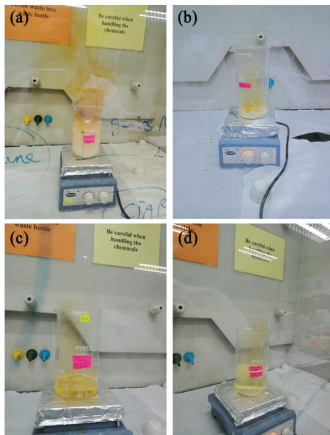
Fig. 1. Images of combustion phenomena of precursors during heating at 350°C (a) FA, (b) CA, (c) OA, and (d) TA.
