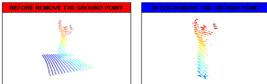
Fig. 4. (left) This figure is taken before removing the ground point; (right) This figure is taken after removing the ground point. Human pose visualization results.
