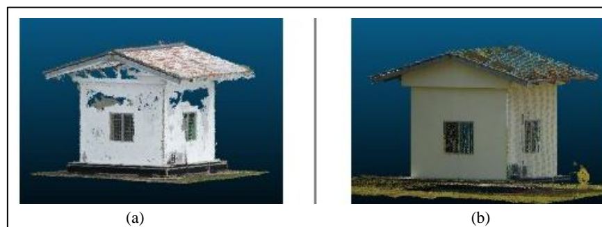
Fig. 5. Overview of the 3D point clouds of the building, (a) UAV, (b) TLS
