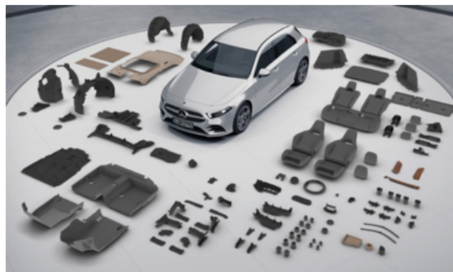
Figure 1. Model of the Mercedes-Benz A-class car and its component parts made of natural fibre composite
