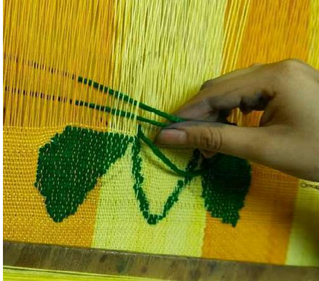
Figure 6. Inlay Technique on tie and dye woven (Source: Student's collection, Nur Insyirah Isa, 2024)
