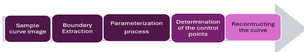
Figure 1: The process of curve construction
