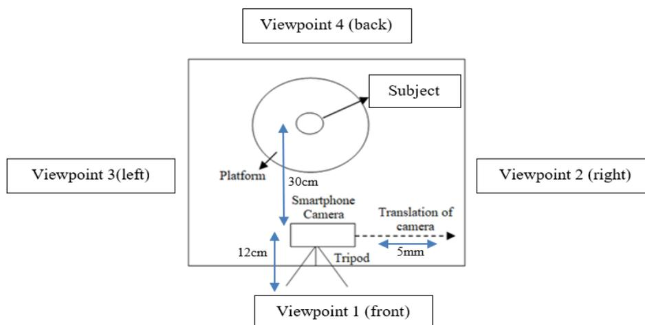
Figure 2: Image Acquisition Set Up
