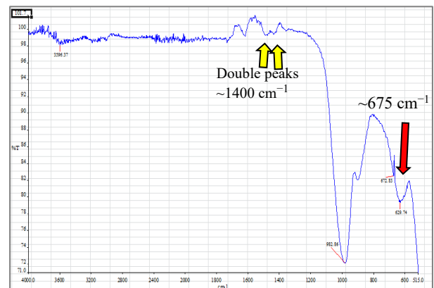
Fig. 7: FTIR spectra for precipitates formed in 940Si:940 Mg at room temperature (Test Condition 3)
