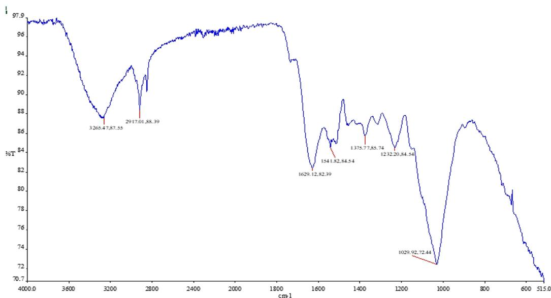
Fig. 3: The FTIR spectrum of areca nut husk
