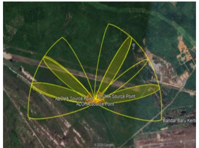
Fig. 6: Area affected from 10 mm diameter leakage (multibed reactor)
