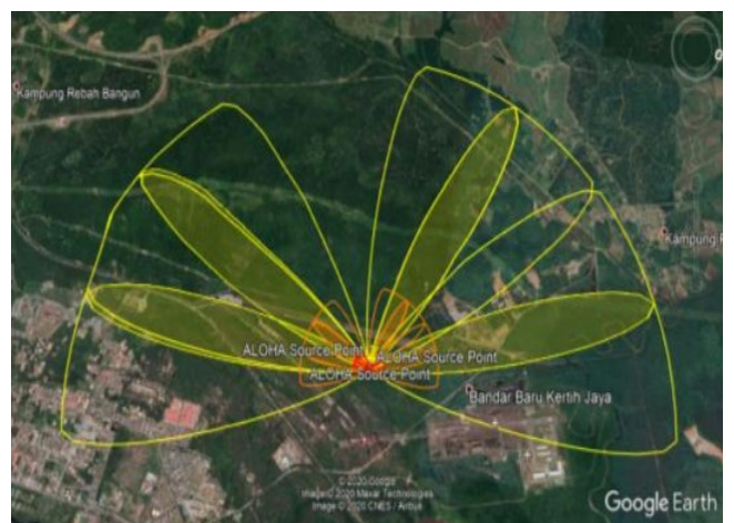
Fig. 8: Area affected from 150 mm diameter leakage (multibed reactor)
