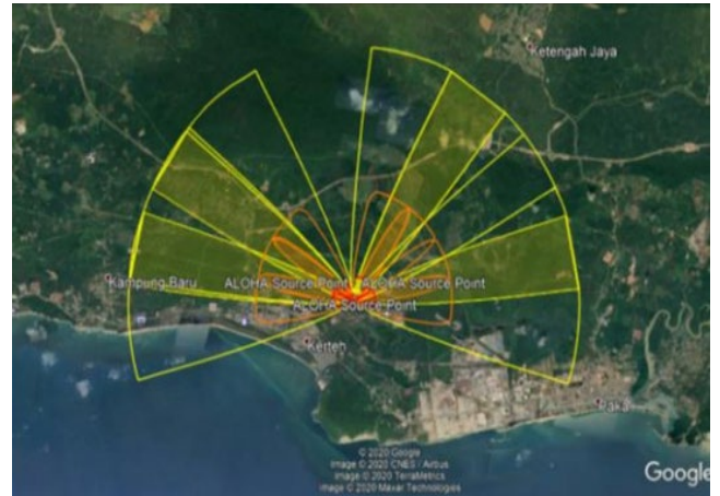
Fig. 9: Area affected from 10 mm diameter leakage
