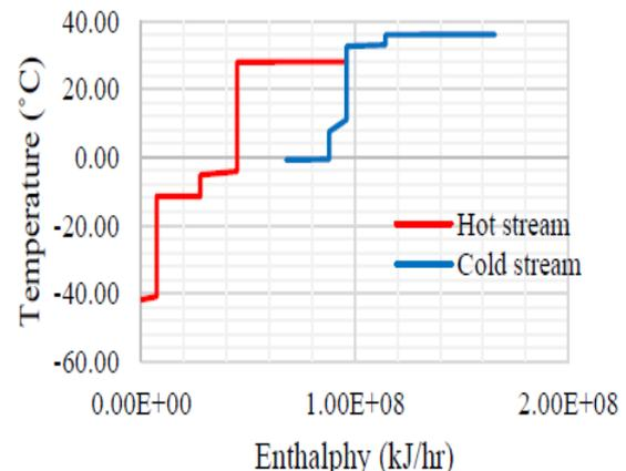
Fig. 5: Composite curve for driving force sequence
