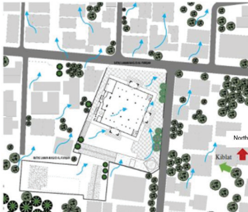
Figure 11. Illustration of Air Flow in the Mosque Environment
