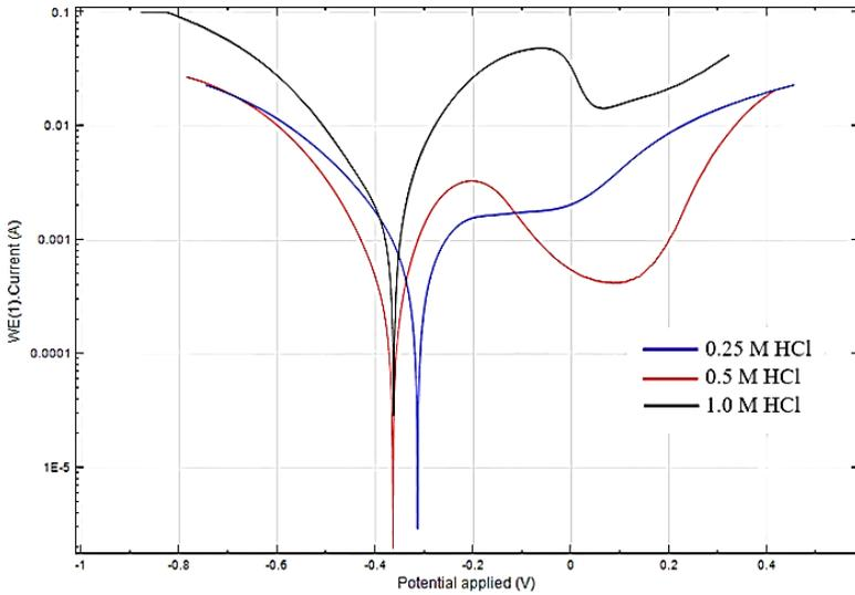
**Figure 5: Tafel polarization curve of SUS304 in 1.5 g/L glycine in different concentrations of HCl**
