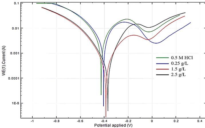
**Figure 4: Tafel polarization curve of SUS304 in 0.5 M HCl and with soybean at different concentration**
