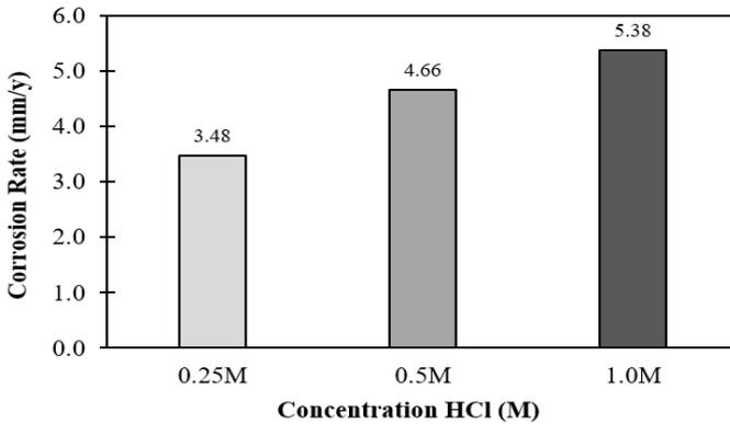
**Figure 2: Corrosion rate of SUS304 in different concentration of hydrochloric acid**
