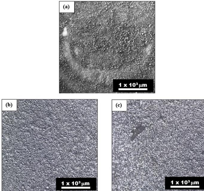
**Figure 6: Optical image of stainless steel SUS304 after immersion test in (a) 0.5 M HCl and with addition of corrosion inhibitors (b) 1.5 g/L soybean (c) 1.5 g/L glycine**
