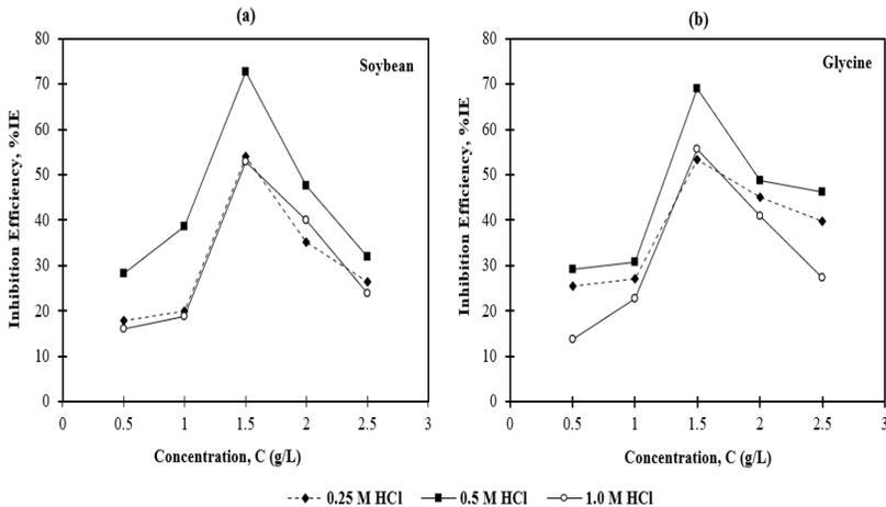
**Figure 3: Corrosion inhibition efficiency (%IE) of SUS304 in different concentration of hydrochloric acid in the presence of (a) soybean and (b) glycine via weight loss method at room temperature  $\pm 25$  °C.**
