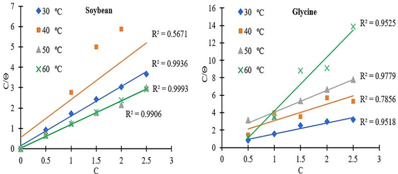
**Figure 7: Langmuir adsorption isotherms for the soybean and glycine adsorbed on the stainless steel surface in 1 M HCl solution at different temperature**
