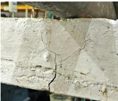
Figure 10: Crack Pattern of Failed Three-Ribbed Slab (source by author)
