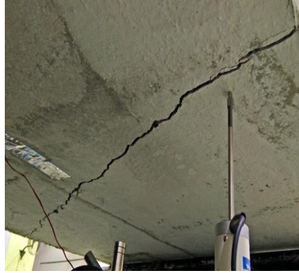
Figure 8: Crack Pattern of Failed Control Slab (source by author)
