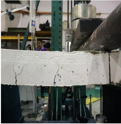
Figure 8: Crack Pattern of Failed Control Slab (source by author)
