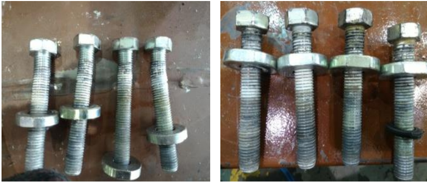
(a) (b) Figure 14: Deformation of Bolts After Test (source by author)
