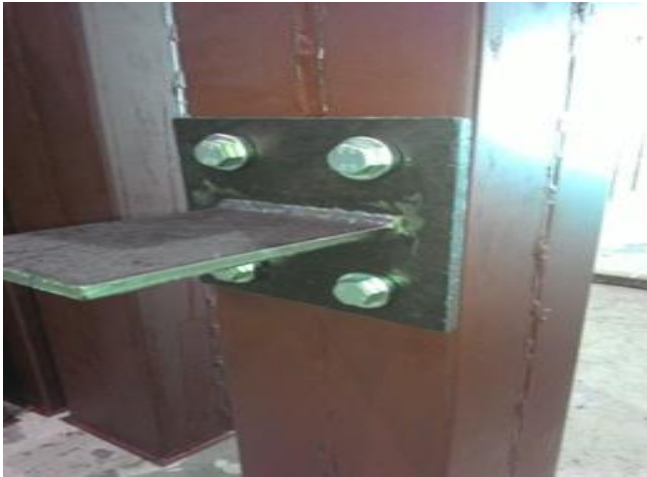
Figure 7: Completed Assemblage of T-Stub End Plate to the CFST using Hollo-Bolt (source by author)
