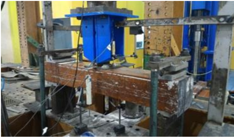
Figure 9: Overall Setup for the Pull-Out Experiment (source by author)
