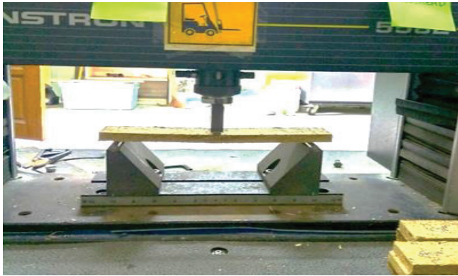
Figure 2: Three-Point Bending Test of Kenaf Particleboard (Source by author)
