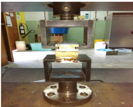
Figure 3: Experimental Set-Up of Internal Bonding Test (Source by author)
