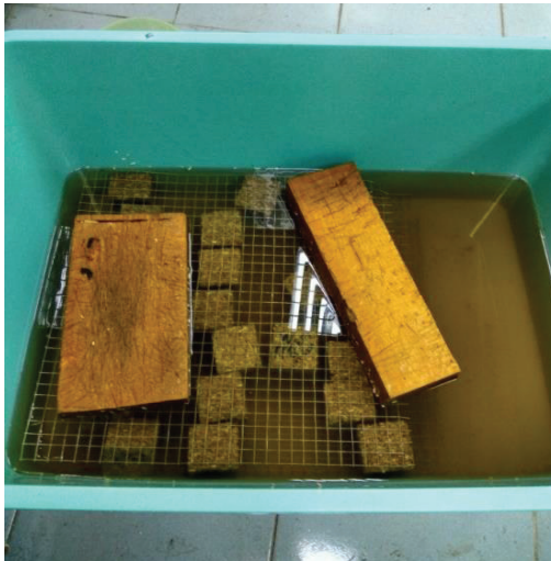
Figure 4: Water Absorption and Thickness Swelling Test (Source by author)
