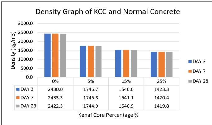
**Figure 6: Density graph of kenaf core concrete and normal concrete**
