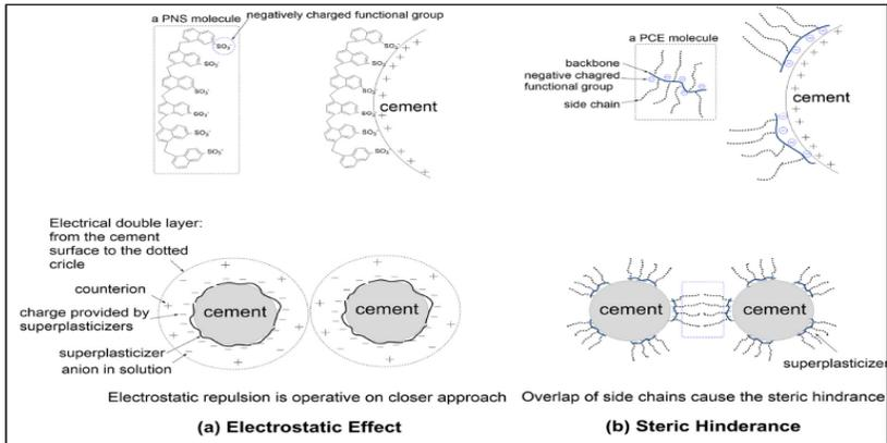
**Figure 1: Schematic illustration of electrostatic repulsion and steric hindrance [10]**
