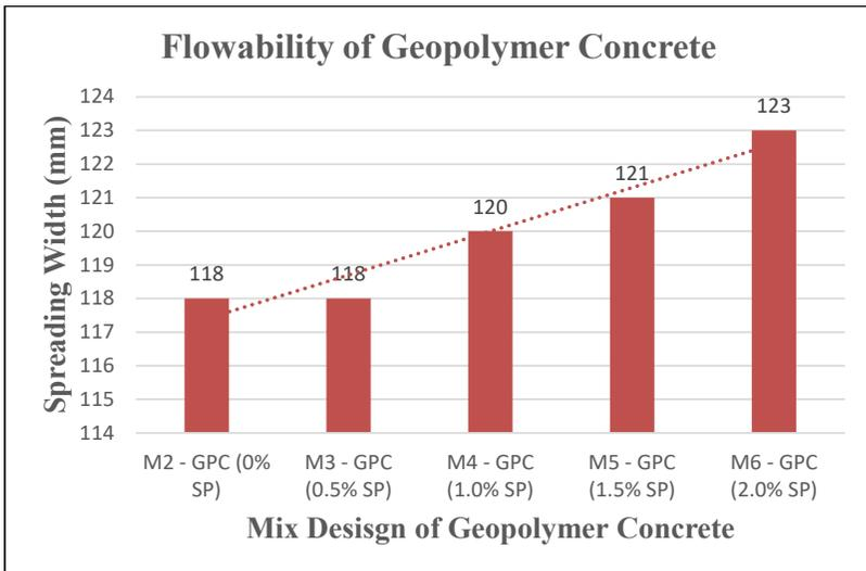
**Figure 8: Flowability of Geopolymer Concrete**
