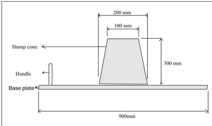
Figure 2: Schematic Diagram of Slump Flow Test Equipment
