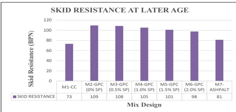
Figure 7: Bar Chart of Skid Resistance at Later Age (28 Days Curing)
