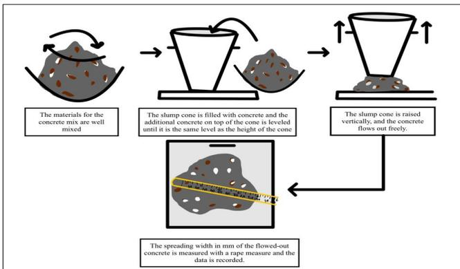
Figure 3: Schematic Diagram for Slump Flow Test Procedure
