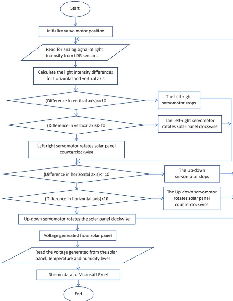
Figure 2: Flowchart of Dual-axis Solar Energy Tracking and Monitoring System
