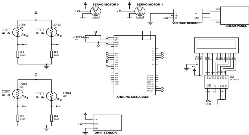
Figure 3: Schematic diagram of Dual-axis Solar Energy Tracking and Monitoring System
