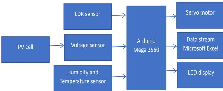
**Figure 1: Block diagram of Dual-axis Solar Energy Tracking and Monitoring System**
