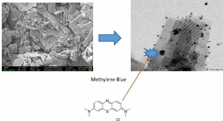
Figure 4: Micrograph (SEM and TEM) of Natural Zeolite-Based Silver and Magnetite Nanocomposites (Source by Kuntubek et al. [75])
