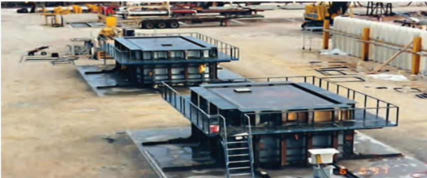
Figure 4: The use of automated steel formwork machine to produce concrete monolith building system (Green Precast Modular System & Technology, 2015)
