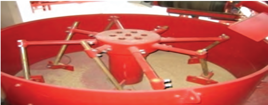
Figure 12: Mechanical arms machine to mix the materials to make the roof tiles (Respondent C)
