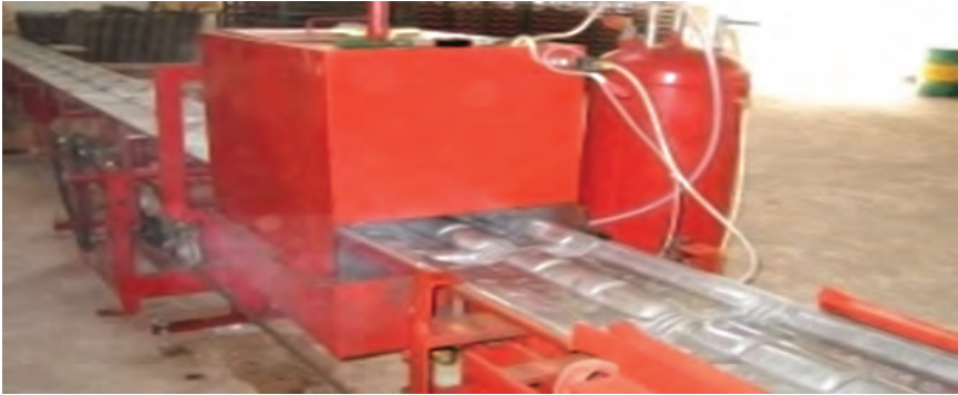
Figure 11: Automated mould oil applicator machine to the roof tile moulds (Respondent C)
