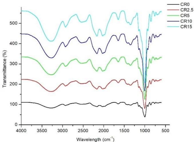
Figure 2: FTIR Spectrum of Starch Film with different CR Compositions
