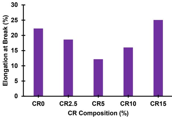
Figure 7: Elongation at break result of films with various CR composition
