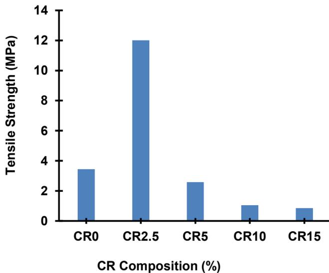
Figure 5: Tensile strength result of films with various CR composition
