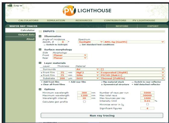
Figure 3: Online simulation Wafer Ray Tracer by PV Lighthouse.
