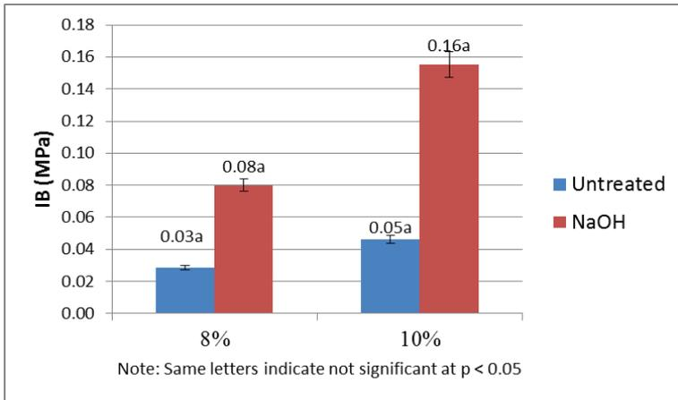
**Figure 3: Effect of resin content on internal bonding test**
