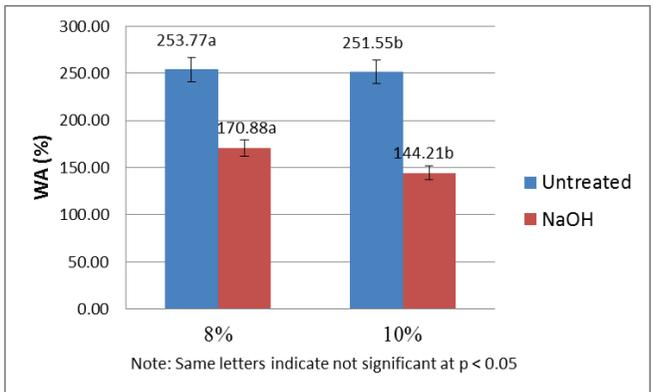
Figure 5: Effect of resin content on water absorption
