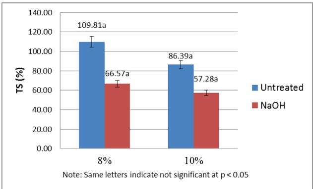
Figure 4: Effect of resin content on thickness swelling
