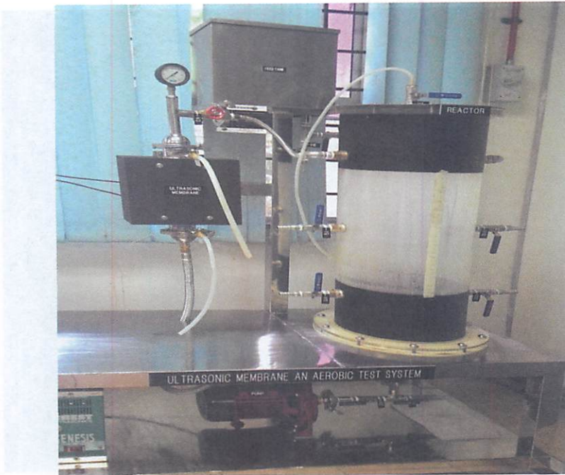
Figure 2: Membrane Anaerobic Reactor (MARS) System in Environmental Laboratory
