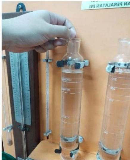
Figure 3: Dropping the steel ball into viscometer
