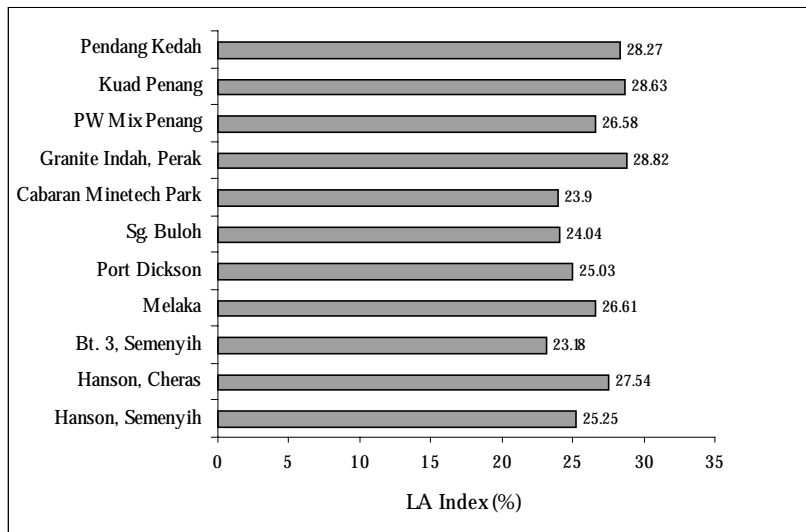
Figure 4: Los Angeles Abrasion Results of Aggregates
