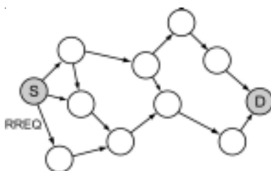
Figure 1: Source Node S Initiates the Path
