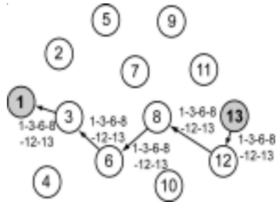
Figure 4: Propagation of Route Reply
