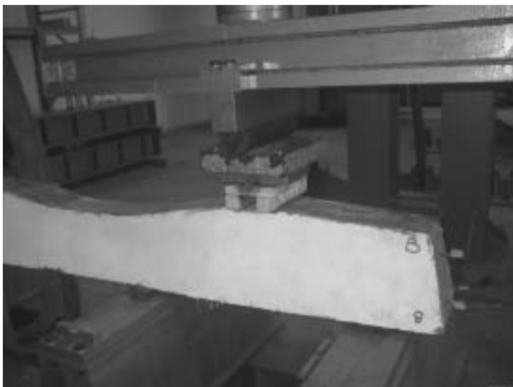
Plate 4: Rail Seat Positive Moment Test Set-up
