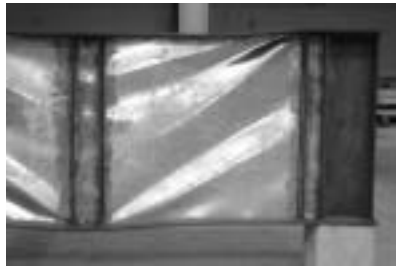
c) Buckling Mode of Specimen F550-1
