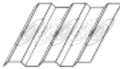
Figure 6b: Zonal Buckling Mode
