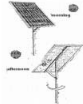
Figure 4: Manual Tracking System using a Rotatable Pole Mount [1].
