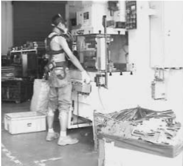
Figure 4: Worker Feeds the Material into Machine Die
