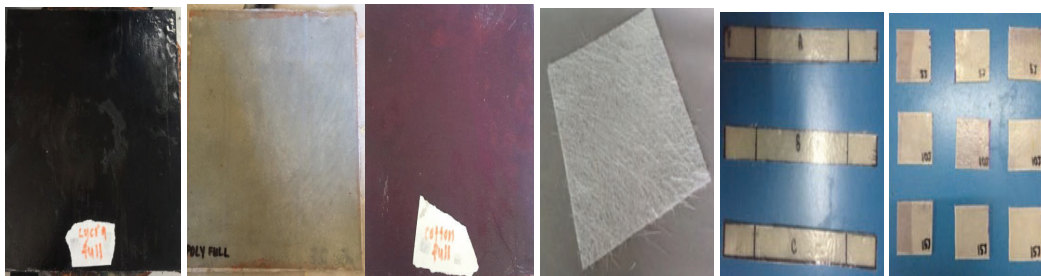
Figure 1: a) Lycra Fabric, b) Polyester Fabric, c) Cotton Fabric, d) Fibreglass e) Samples for Tensile Testing f) Samples for Impact Testing
