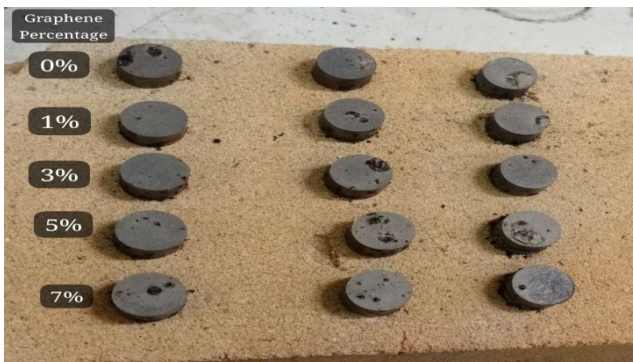
Figure 2: Fabrication of Mg-Zn alloy reinforced with graphene.
